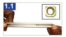
Insert 2\*M5 Nuts into the LNB Mounting Rail;
