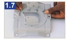
Place and tighten the Rotation Bracket onto the Reflector Back Mount using 3\*M6x12 Hexagonal Flange Bolts;
