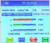
Fine tune reflector pointing for elevation (up/down) and azimuth (East/West) angles producing optimal signal strength & quality.
