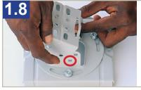
Place and tighten the Elevation Bracket onto the Rotation Bracket with 4\*(M6x12 Carriage Bolts+M6 Nuts);
