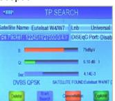
Fine tune LNBF Clamp position on LNBF Mounting Rail, as well as LNB mounting angle, as well as Reflector rotation to optimize signal strength & quality. Preceding steps to be repeated in the same sequence, until optimal results are achieved. When done, verify that the 16A signal values have not been adversely affected. If necessary, redo 3.1. Record both 16A and 36A/B resulting readings;
