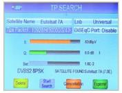
Fine tune LNBF Clamp position, as well as LNBF mounting angle to optimize signal strength & quality. Preceding steps to be repeated in the same sequence, until optimal results are achieved. When done, verify that the 16A and 36A/B signal values have not been adversely affected.
